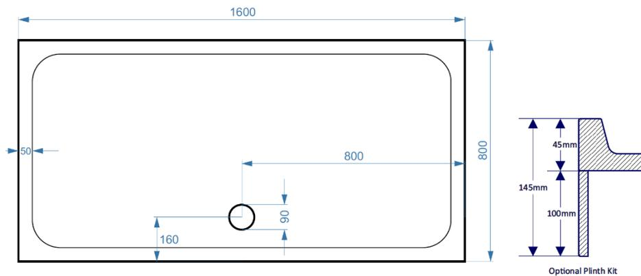
All measurement stated in mm to tolerance of +-5mm
