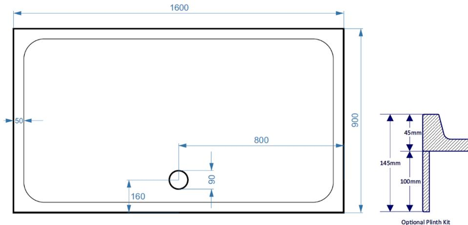
All measurement stated in mm to tolerance of +-5mm
