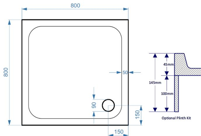
All measurement stated in mm to tolerance of  $\pm 5$ mm
