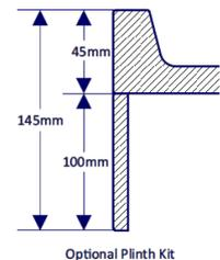
All measurement stated in mm to tolerance of +-5mm
