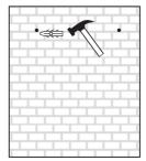
2. Drill the holes in the wall for the screw plugs supplied in the fixing kit. Ensure the holes are horizontal using a spirit level. Fasten the screws into the plugs leaving the screw head protruding about 10-8mm from the wall.
