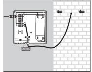
3. Unscrew the lid of the plastic box at the back of the mirror. Use the electrical connections found inside the box to connect the mirror to the main supply in accordance with the current IEE regulations. Once the connection is made, screw the lid back on the plastic box. Hang the mirror on the wall and switch on the electrical supply.
